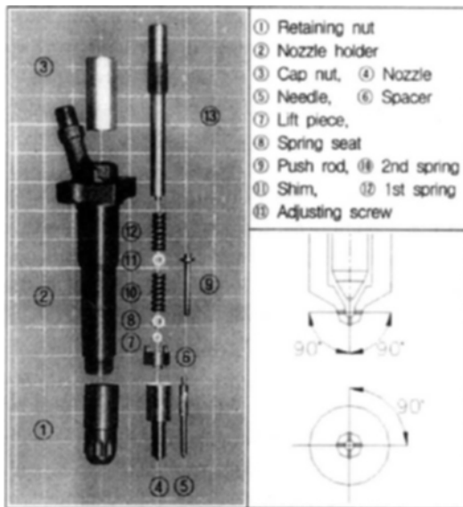
Fig. 2 Photograph of disassembled 5-hole diesel nozzle and schematic diagram of nozzle tip
